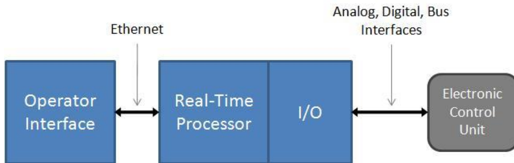
Figure 1. An HIL test system consists of three primary components: an operator interface, a real-time processor, and I/O interfaces.
