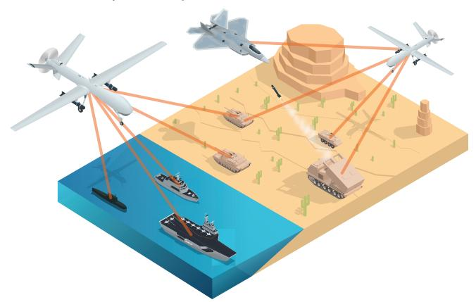
Electronic warfare relies extensively on sensors across the electromagnetic spectrum – signals such as radio, infrared or radar – to provide 360-degree situational awareness and advanced signals intelligence while denying the enemy the opportunity to do the same or to prevent the enemy from disrupting friendly use of the spectrum.
