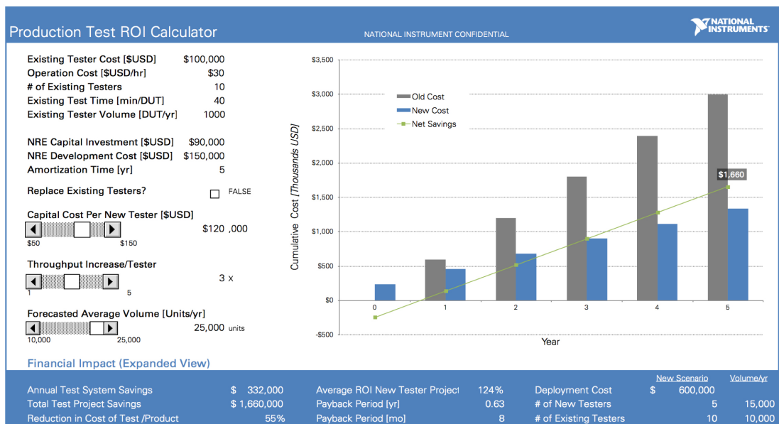
Figure 7. The new test system generates a total savings of $1.66 million in five years with a payback period of 11 months in comparison to scaling up the existing solution.
