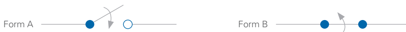
Figure 7. SPST relays come in two forms: normally open (Form A) and normally closed (Form B).
