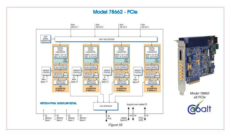
Model 78662 is a member of the Cobalt family of high-performance PCIe boards based on the Xilinx Virtex-6 FPGA. Based on the Model 71660 presented previously, this four-channel, high-speed data converter with programmable DDCs is suitable for connection to HF or IF ports of a communications or radar system.
