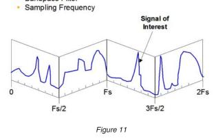
The third sampling mode, called undersampling or subsampling, is ideal for many systems that use an analog RF translator front end. These receivers usually deliver IF outputs, often at 21.4 or 70 MHz, with bandwidths ranging from a few kilohertz to tens of MHz—depending on the receiver.
