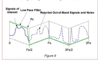
For the baseband wideband sampling mode, where we want to look at everything from DC up to a frequency below the half sampling rate, we can install a low pass filter with a cutoff frequency, Fc, located below Fs/2.
