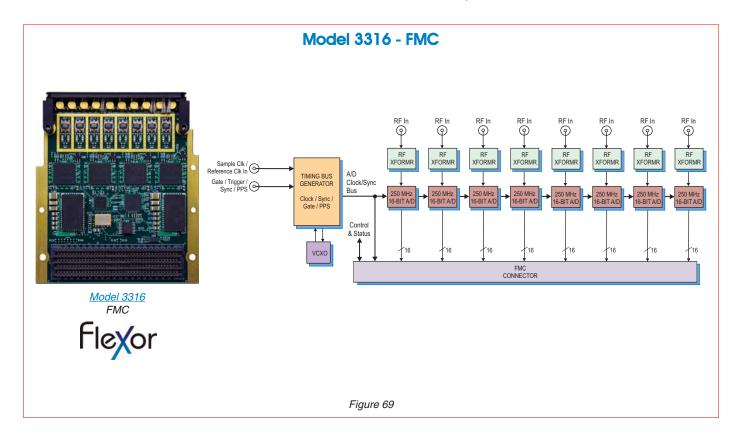
The Flexor Model 3316 is a multichannel, high-speed data converter FMC module. It is suitable for connection to HF or IF ports of a communications or radar system. It includes eight 250 MHz, 16-bit A/Ds, on-board programmable clocking, and multiboard synchronization for support of larger high-channel-count systems.
