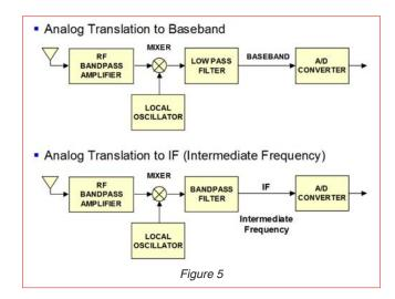
In the case where the antenna signal frequency is too high to be digitized directly by the A/D converter, it has to be translated down using an analog mixer and local oscillator.
