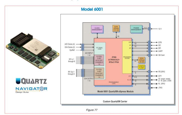
The Quartz Model <u>6001</u> is a high-performance Quartz eXpress Module (QuartzXM) based on the Xilinx Zynq UltraScale+ RFSoC FPGA. The RFSoC FPGA integrates eight RF-class A/D and D/A converters into the Zynq's multiprocessor architecture, creating a multichannel data conversion and processing solution on a single chip.
