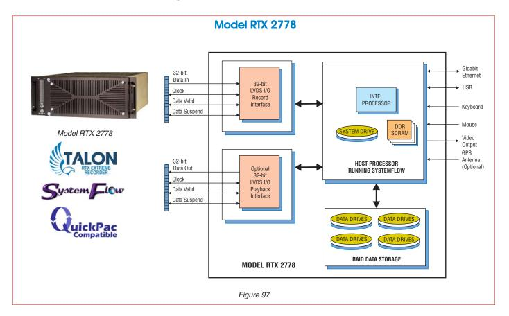
The Talon RTX 2778 is a turnkey record and playback system that is built to operate under harsh conditions. Designed to withstand high vibration and operating temperatures, the RTX 2778 is intended for military, airborne and UAV applications requiring a rugged system.
