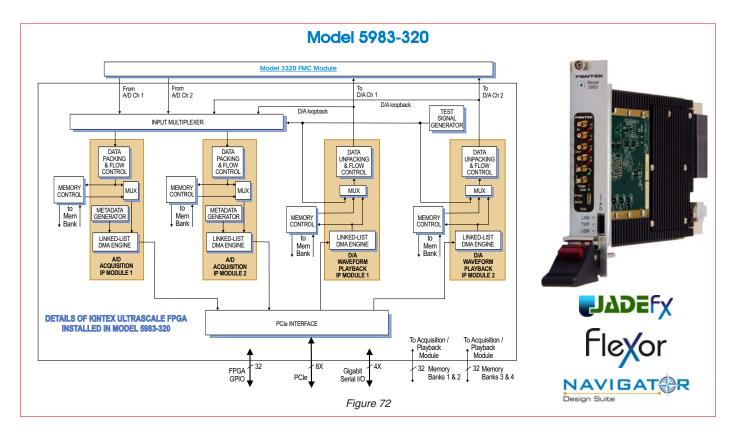
Model 5983 is a member of the JadeFX<sup>TM</sup> family of highperformance 3U VPX baseboards with a Xilinx Kintex UltraScale FPGA and an available FMC I/O slot.
