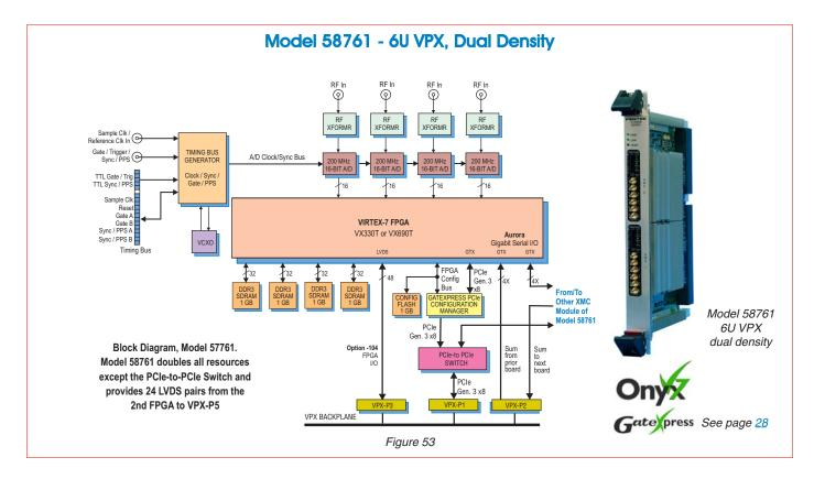
Model 58761 is a member of the Onyx family of high-performance VPX boards based on the Xilinx Virtex-7 FPGA. A multichannel, high-speed data converter based on the Model 71760 described previously, it includes factory-installed IP cores to enhance the performance of the 71760 and address the requirements of many applications.
