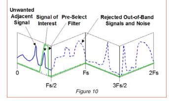
For the baseband **preselect** sampling mode, we need to use a bandpass filter with the frequency response shown in green.
