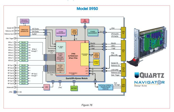
The Quartz<sup>TM</sup> Model <u>5950</u> is a high-performance 3U VPX board based on the Xilinx Zynq UltraScale+ RFSoC FPGA. The RFSoC integrates eight RF-class A/D and D/A converters into the Zynq's multiprocessor architecture, creating a multichannel data conversion and processing solution on a single chip. The Model <u>5950</u> brings RFSoC performance to 3U VPX with a complete system on a board.
