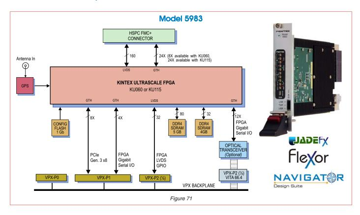
The JadeFX<sup>™</sup> Model 5983 is a high-performance 3U OpenVPX board based on the Xilinx Kintex UltraScale FPGA. As a stand-alone processor board, it provides an ideal development and deployment platform for demanding signal-processing applications.
