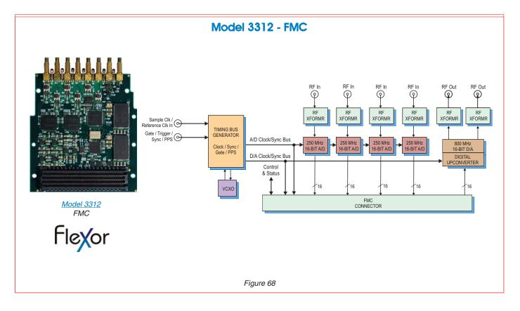
The Flexor Model 3312 is a multichannel, high-speed data converter FMC module. It is suitable for connection to HF or IF ports of a communications or radar system. It includes four 250 MHz, 16-bit A/Ds, two 800 MHz, 16-bit D/As, programmable clocking, and multiboard synchronization for support of larger high-channel-count systems.
