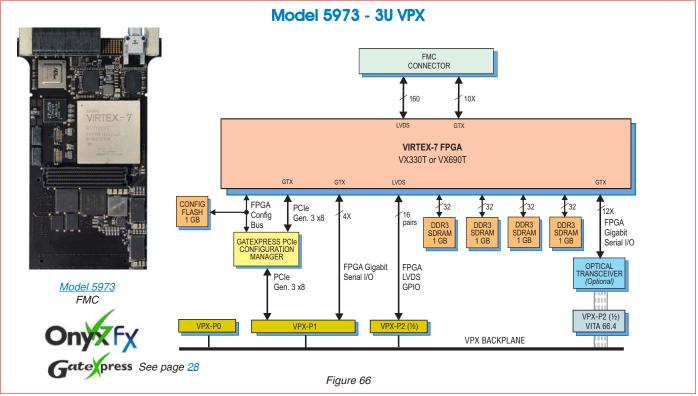
The OnyxFX<sup>TM</sup> Model <u>5973</u> is a high-performance 3U VPX board based on the Xilinx Virtex-7 FPGA. As a stand-alone processor board, it provides an ideal development and deployment platform for demanding signal-processing applications.
