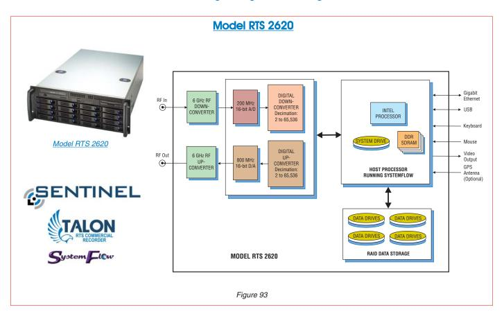
The Talon RTS 2620 combines the power of a Pentek Talon Recording System with those of an RF tuner and RF upconverter hardware plus Pentek's Sentinel Intelligent Signal Scanner. The RTS 2620 provides SIGINT engineers the ability to scan the 6 GHz spectrum for signals of interest and monitor or record bandwidths up to 40 MHz wide once a signal band of interest is detected.
