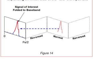
The effect of undersampling, as you probably expected by now, is that the IF signal is folded down to the first page. This is really an automatic frequency translation, performed for free by the sampling process.
