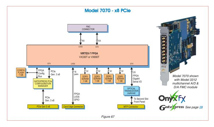
The OnyxFX Model <u>7070</u> is a high-performance PCIe board based on the Xilinx Virtex-7 FPGA. As a stand-alone processor board, it provides an ideal development and deployment platform for demanding signal processing applications.
